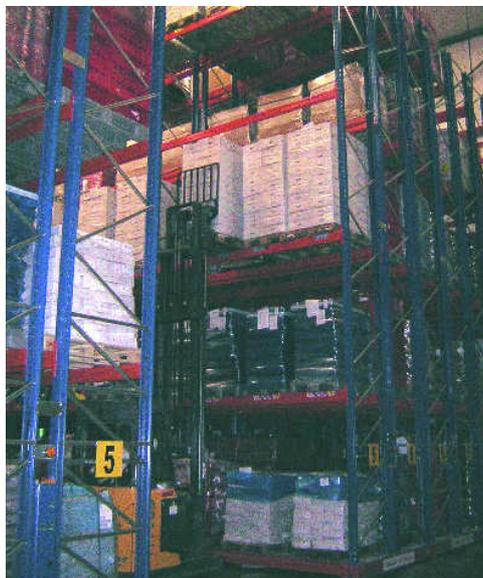
An automated sliding rack is operated over five levels on two fixed racks with 16 racks on mobile carriages via remote control from the lift truck.
